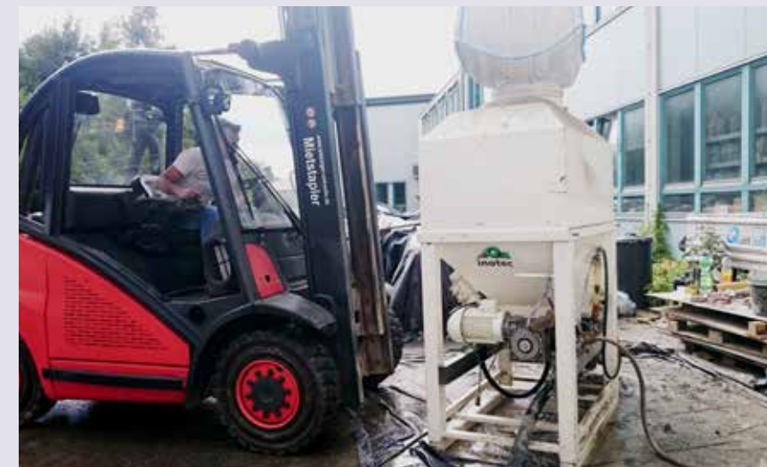
Two Big-Bag-Boxes Mono in combination with the inoFLEX Duo for indirect filling with big bags
