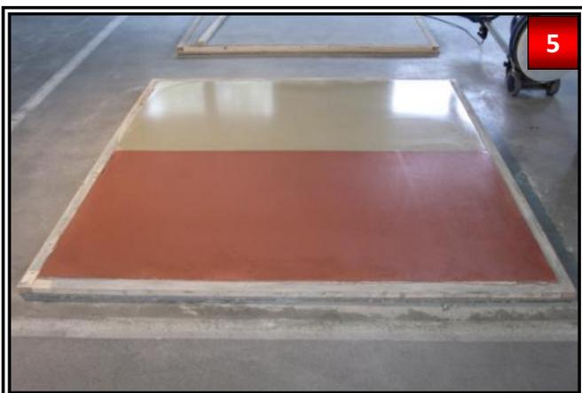
OBTEGO® R-400 penetrates largely into the floor surface. A slightly, oily smear film remains on the surface.
